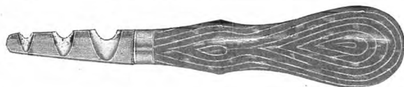
No. 903 Safety Edger, Style A, heavy Sizes 00-0-1-2-3-4-5-6
